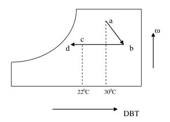
Locate point 'a',  $30^{0}$ C DBT, 50% RH, the atmospheric condition. Locate point 'c',  $22^{0}$ C DBT, 60% RH, the required indoor condition. "Since chemical dehumidification process follows constant enthalpy line" at a draw a line parallel to constant enthalpy line.
