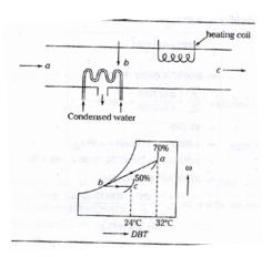
Locate point 'a' 32°C, 70% RH out door condition Locate point 'c' 24°C DBT, 50% RH required condition At c draw a horizontal line to cut the saturation line at point 'b' Join ab  $ab \rightarrow$  cooling and dehumidification  $bc \rightarrow$  heating
