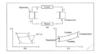
*Expression C.O.P when compression and expansion are Isentropic* Refrigeration Effect = Heat removed from the refrigerator
