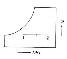
At 40°C DBT  $P_{VS} = 0.07375bar$ During sensible heating  $\omega$  and  $p_v$  remain constant  $p_v = 0.0284bar$   $RH = \phi = \frac{p_v}{p_{vs}} = \frac{0.0284}{0.07375}$  = 0.385 = 38.5%  $H_2 = 1.005x40 + 0.0179(2500 + 1.88x40)$  = 86.29kJ/kg of dry air Weight of 300m<sup>3</sup> / min of air  $= \frac{(p - p_v)V}{RT}$   $= \frac{(1 - 0.0284)x300x10^2}{0.287x303} = 335.18kg / min$   $\therefore$  Heat added/min = 335.18(86.29 - 76) = 3449kJ/min From chart WBT = 27.2°C
