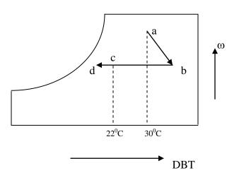
Locate point 'a',  $30^{0}$ C DBT, 50% RH, the atmospheric condition. Locate point 'c',  $22^{0}$ C DBT, 60% RH, the required indoor condition. "Since chemical dehumidification process follows constant enthalpy line" at a draw a line parallel to constant enthalpy line.
