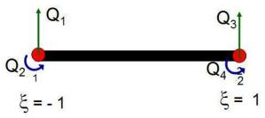
The shape functions of beam element are called as Hermite shape functions as they contain both nodal value and nodal slope which is satisfied by taking polynomial of cubic order
