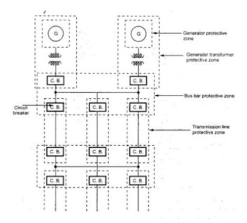
The boundaries of protective zones are decided by the locations of the current transformer. In practice, various protective zones are overlapped. The overlapping of protective zones is done to ensure complete safety of each and every element of the system. The zone which is unprotected is called dead spot. The zones are overlapped and hence there is no chance of existence of a dead spot in a system. For the failures within the region where two adjacent protective zones are
